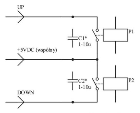
the elevator can operate in monostable mode (closing the circuit for a time longer than about 1 s) or bistable mode (closing the circuit for a time shorter than about 1 s)
