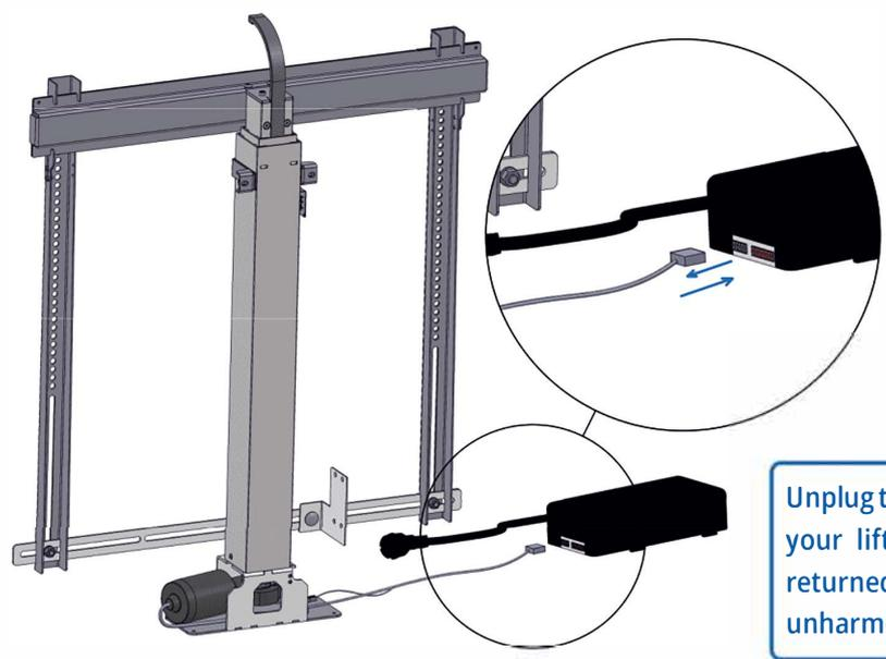
**Unplug the original control box from your lift. The control box can be returned for a refund, if delivered unharmed.**
