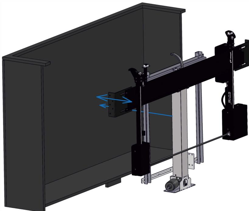
Autolid is delivered with 2 sets of adjustable brackets to be fixed on the sides of the furniture. Use them according to your TV dimensions.
