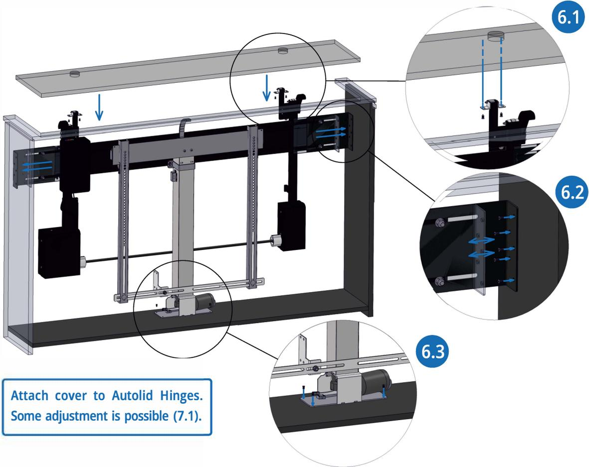
Attach cover to Autolid Hinges. Some adjustment is possible (7.1).
